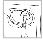
2. Connect the other end of the water inlet hose to the washerdryer, screwing it onto the appliance's cold water inlet, situated on the top right-hand side on the rear of the appliance (see figure).
